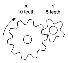
Gear **X** is rotated clockwise at 1.0 rotation per second.
