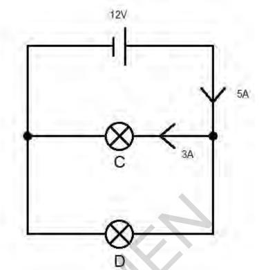
Use the formula **resistance = potential difference ÷ current** to calculate the resistance of bulb **D**.
